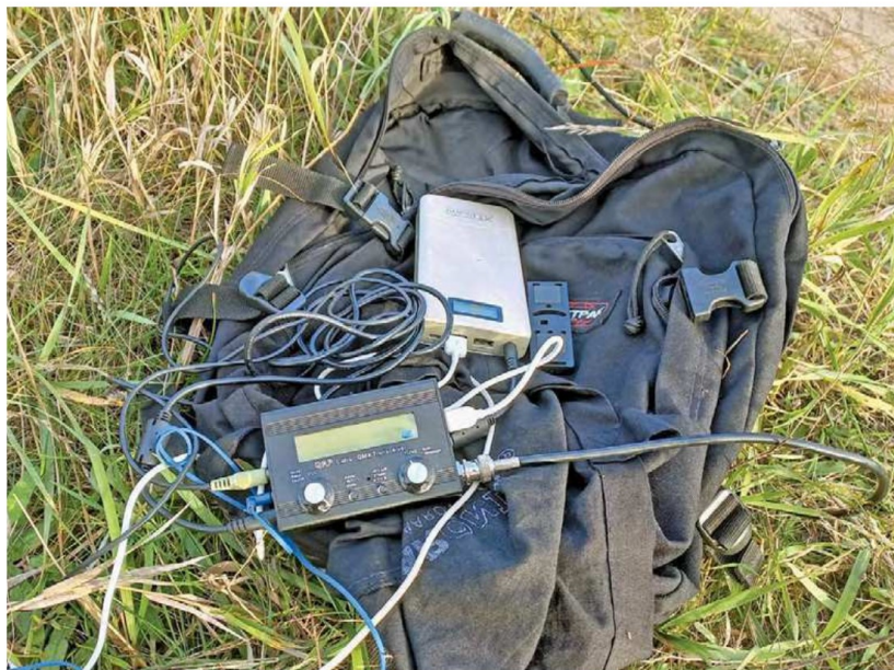
Andrea Borgnino, IWØHK, used his small POTA kit (a QMX transceiver, a 20-meter end-fed half-wave antenna, and an XTPower XT-16000QC3 power bank) for the first time during his Berlin activations, which were a success.
